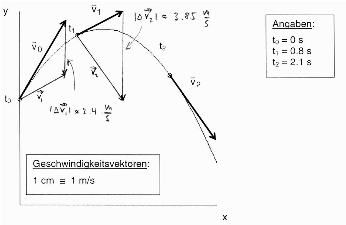
$$b.) \quad |\vec{a}_1| = \frac{|\Delta \vec{v}_1|}{\Delta t} \Rightarrow |\vec{a}_1| = \frac{2.4 \text{ m/s}}{0.8 \text{ s}} = 3 \frac{\text{m}}{\text{s}^2}$$
